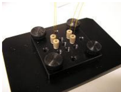
Figure A.2-3. The chipholder in which the nanoslit device is fixed. The connectors can be screwed into the chipholder and connect the device to the syringes and buffer vials.
